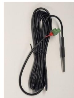
Figure 101. Renogy remote temperature sensor.
