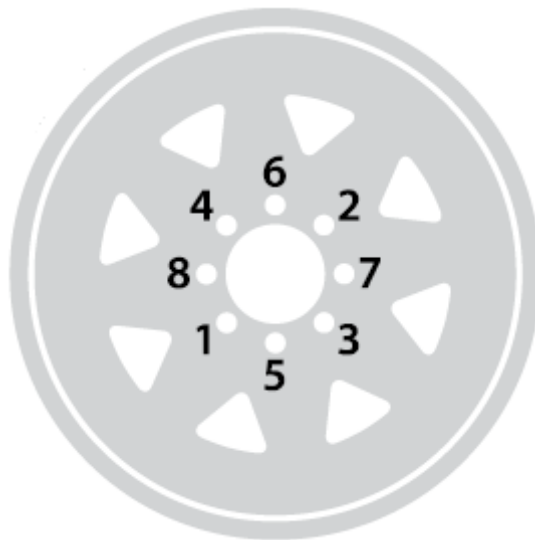
Figure 4. Proper lug nut torque sequence for an eight-lug wheel.
