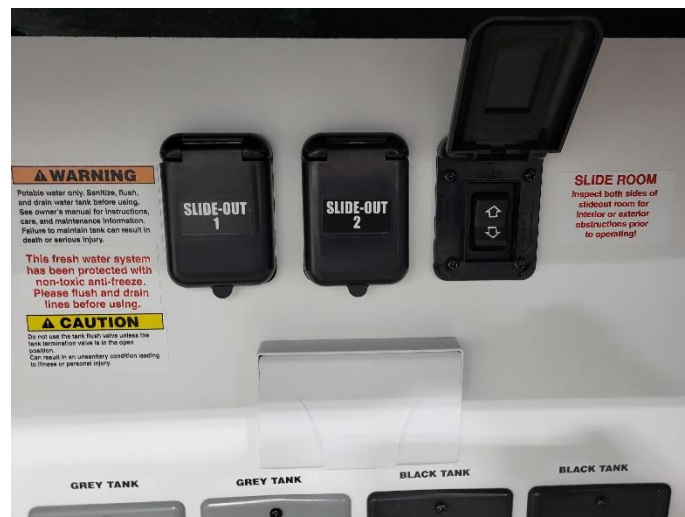
Figure 40. Remote slide controls in the utility bay of the Paradigm.
