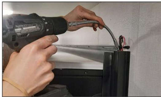
Figure 64. Using the flexible drive tool to manually override the slide.
