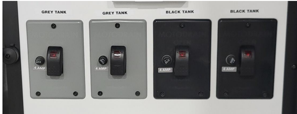
Figure 147. Electric waste valve actuator switches in the utility bay.
