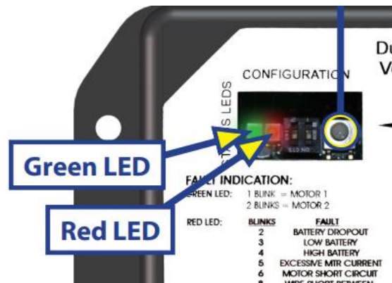
Figure 60. Controller indicator LEDs.
