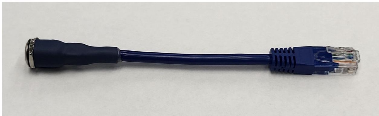
Figure 68. Renogy battery activation cable.
