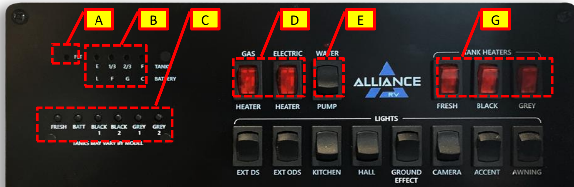
Figure 150. The upper portion of the monitor panel showing tank and water controls. This figure has the same indicators as Figure 121.
