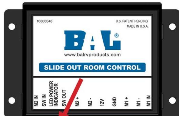
Figure 63. BAL Exact-Slide controller, with indicator lights shown in lower left corner.
