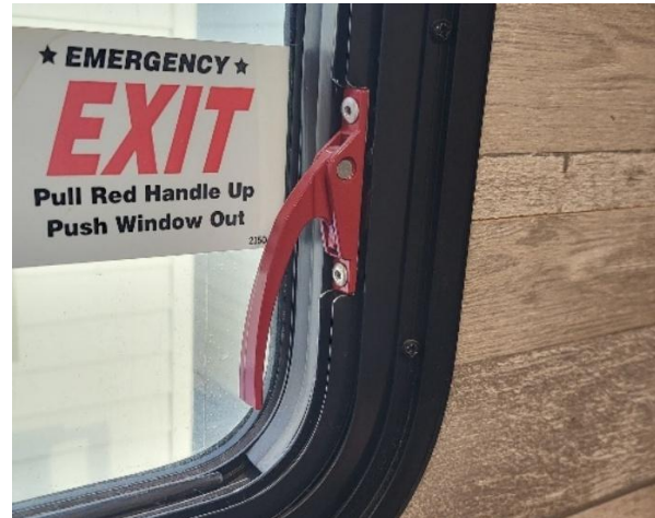
Figure 28. Pull-Lever style latch on an emergency exit. Pull the leverl out, away from base, to disengage latch. Push window out.
