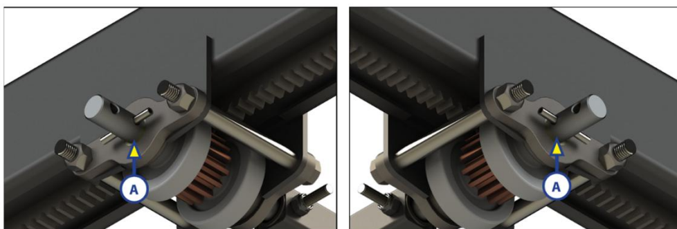
Figure 47. Gear Pack lubrication points - exterior.
