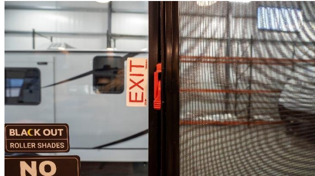
Figure 25. Tab style latch on an emergency exit.
