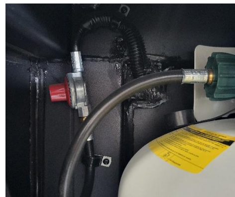
Figure 32. Step down propane regulator for long hose lengths, dropping pressure from tank levels to 30 psi.
