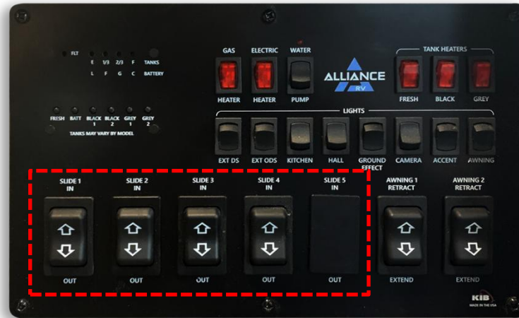
Figure 39. Monitor panel with slide-out controls highlighted.
